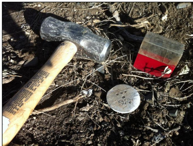
Figure 1: Control point set in concrete and labeled
