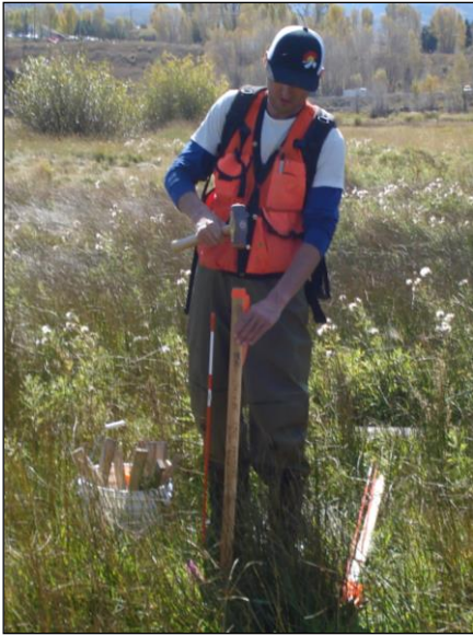
Figure 2: Mark rebar pins with lathe or t-posts, flagging, and record their coordinates with a GPS. Building a small rock cairn around the pin can also be useful for relocating them in the future.
